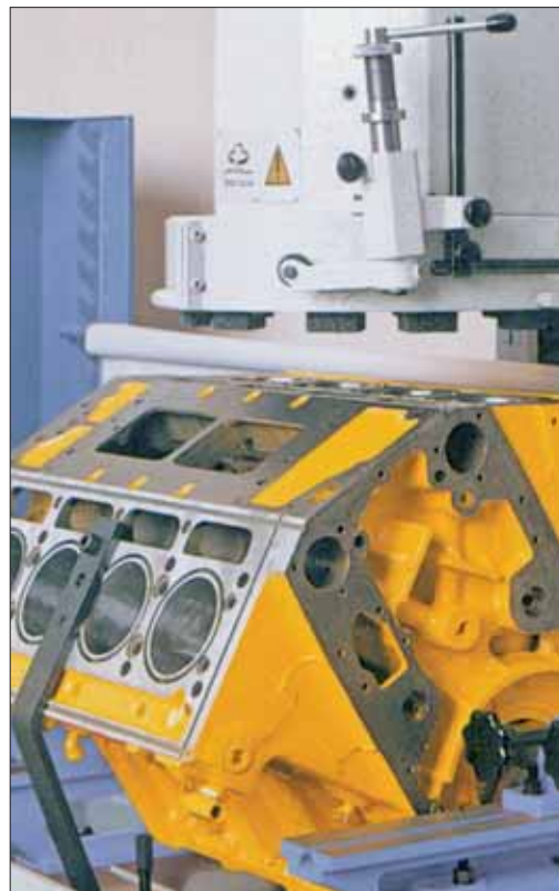
Fig. 14 Piazzamento inclinabile per testate motori a "V". Slanting setup fixture for "V" - type cylinder heads.
