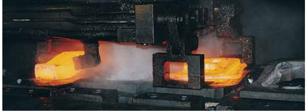
Track links forging
