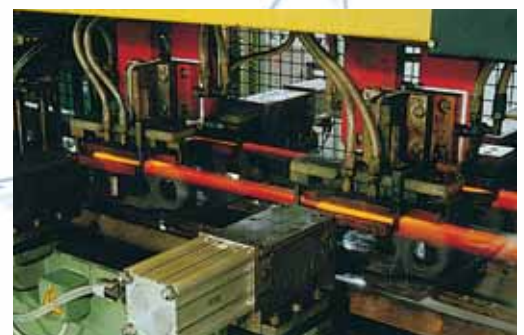
Induction hardening of track links
