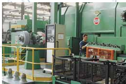
Split master links creep feed grinding
