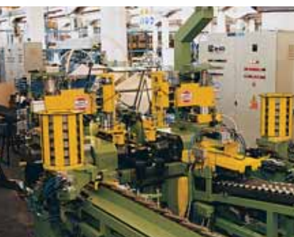
▼ Track chains fully automated assembly
