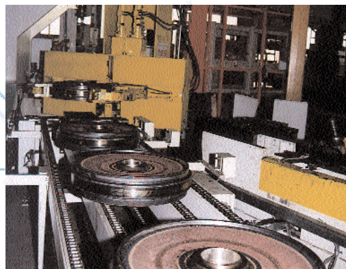
FMS line for automated assembly of Idler Groups
