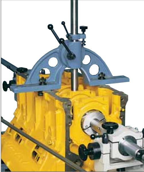
Fig. 7 Setting up a V-block; one can see the central support for the boring bar. The special lock clamps are available on request, at extra cost.
