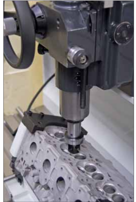
Fig. 1 Removing worn valve seat ring and chambering for new ring
