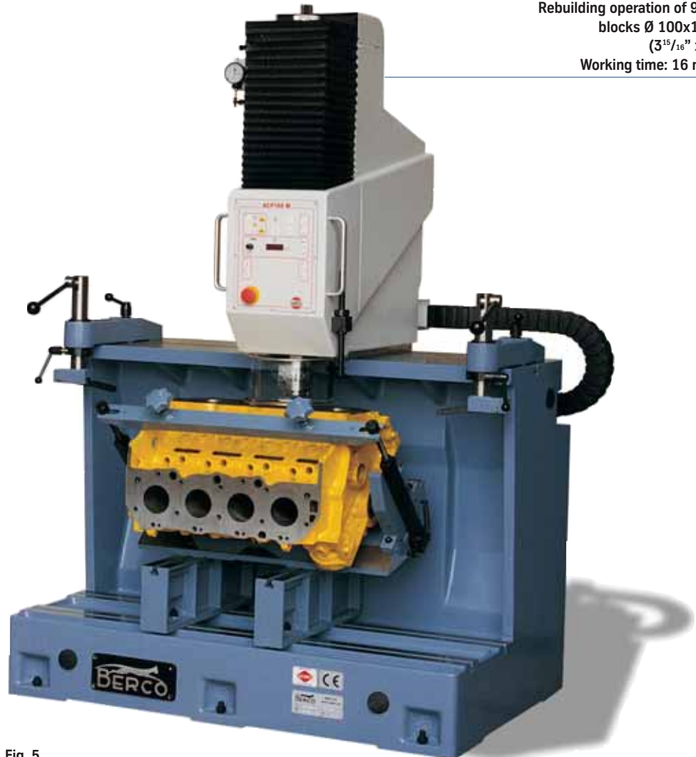
Fig. 5 ACP160M set up for reconditioning "V" 90° blocks.
